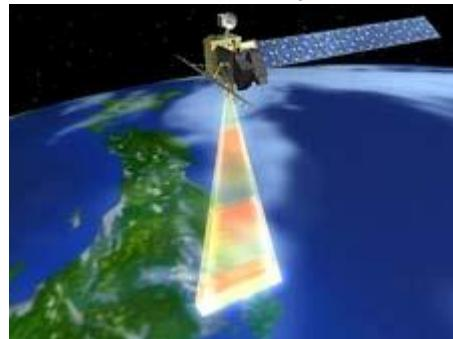
AVNIR-2 can observe with 10m resolution in 70km swath, and it can be changed the observation area by pointing capability within +/-44 deg. in across track.
