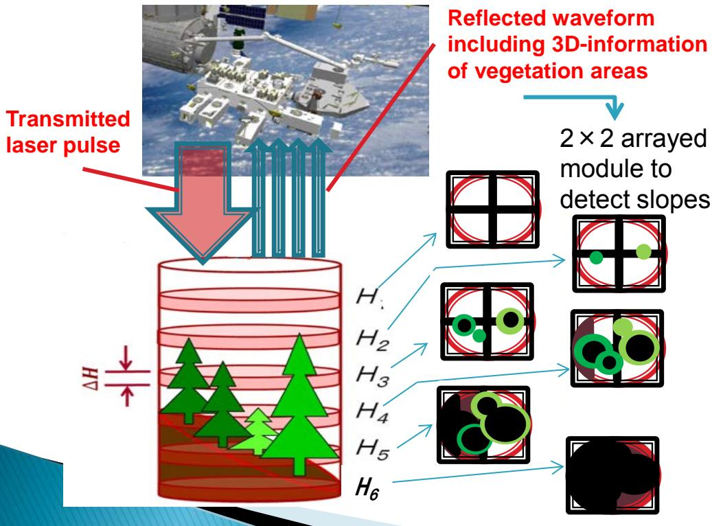
Schematic diagram of the vegetation lidar mission.
