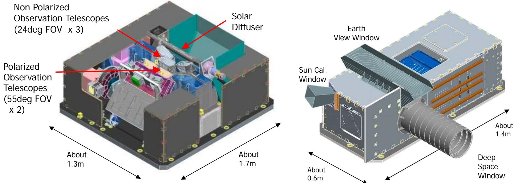
Visible and Near Infrared Radiometer
