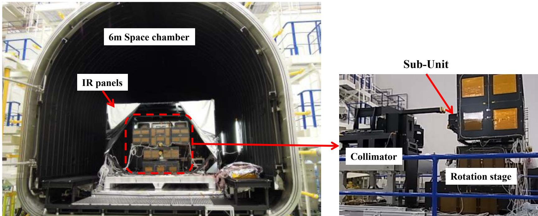
Collimator and Rotation stage are setting in the 6mφ Space chamber in TSUKUBA
