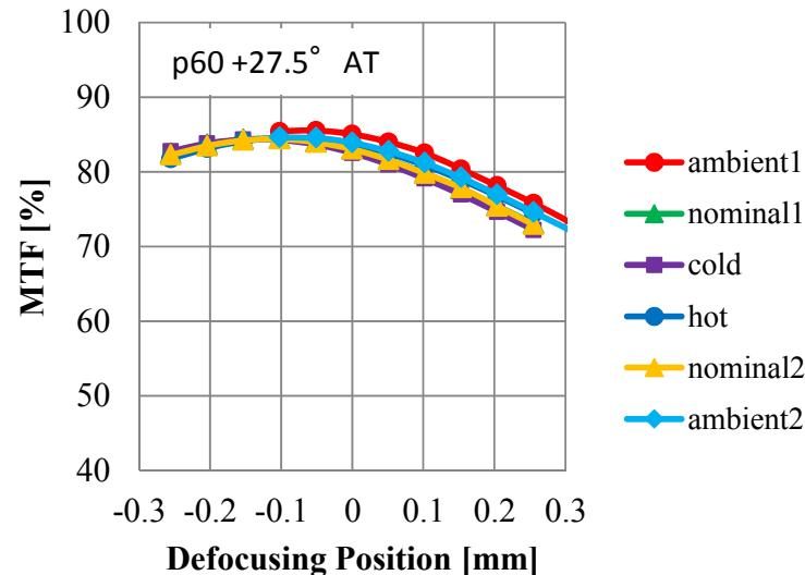
The ambient data are the corrected value due to the vacuum shift of focal length
