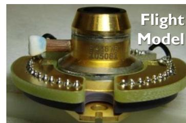
Long Wave Infrared Detector (LWIRD)
