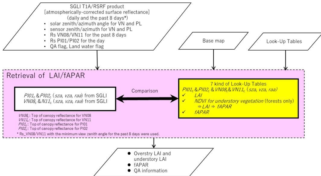
Figure 1. Processing flow
