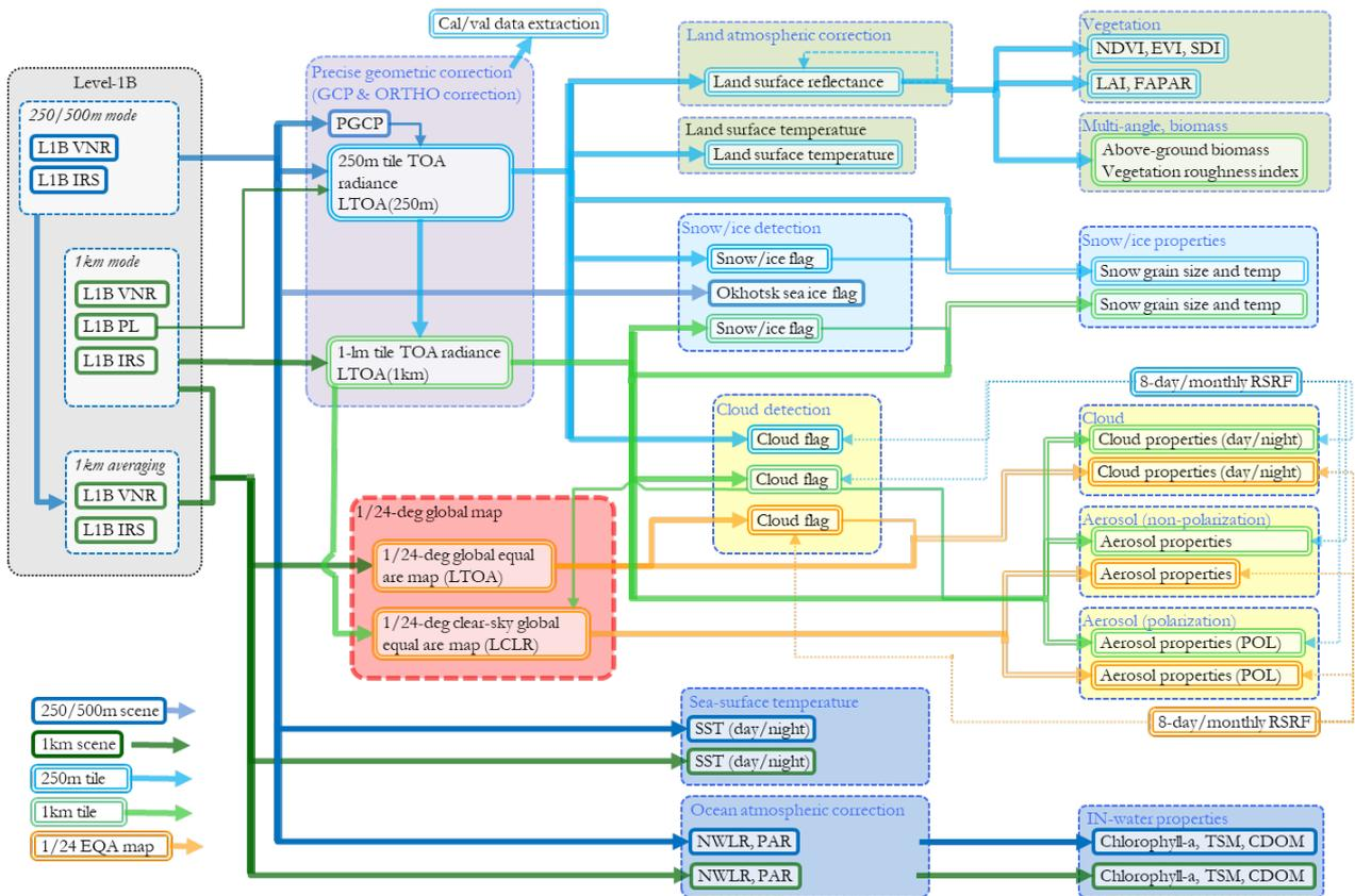
Figure 1 GCOM-C processing flow from Level-1B to Level-2
