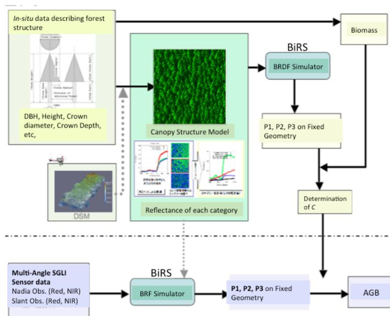
Figure 4. Schematic diagram for AGB estimation.
