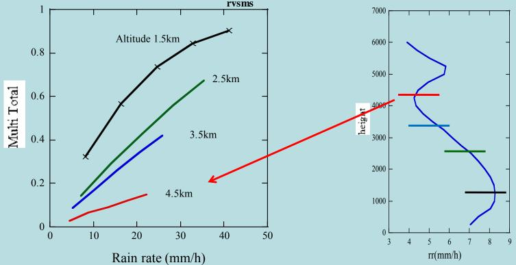
MS contribution increases with rain rate. MS contribution is <u>90%</u> at altitude of 1.5 km. <u>Bias in rain rate?</u>
