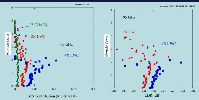
LDR is difficult to measure with ground-based radar at lower frequencies than 35 GHz.But radar at 95GHz may be useful.
