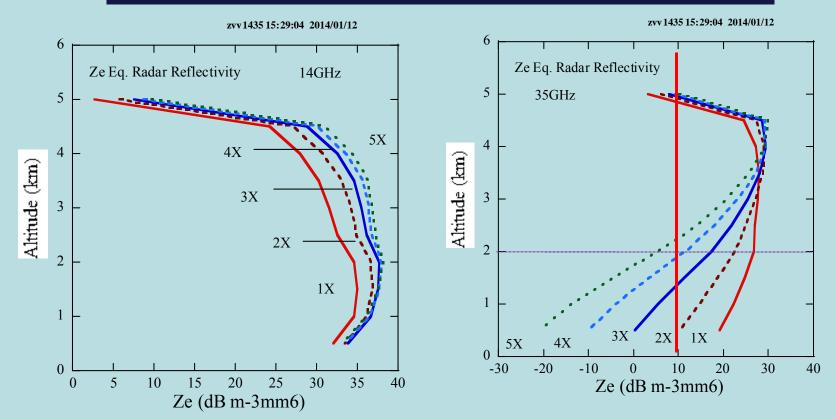
Significant decreases in Ze at 35 GHz. Data at 35 GHz is difficult to detect at lower altitude. MS contribution at 2.5 km is 30% and leads to bias of 15% in rain rate.
