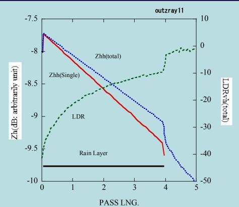
LDR (green) increases with MS contribution. However, no LDR is available in GPM. Use of ground-based radar?
