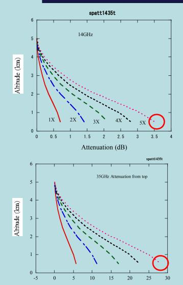
Attenuation is 3.5db at 14GHz 27dB at 35 GHz for model 5x.
