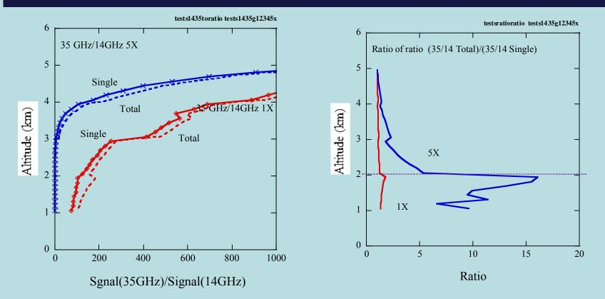
MS effects modified the ratio of received power at 35 GHz and 14 GHz. Data at 35 GHz is difficult to detect at lower altitude. The ratio is about five times at altitude oof 2km for 5x model.
