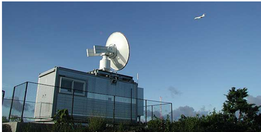
X-band Doppler radar installed in Aimeliik
