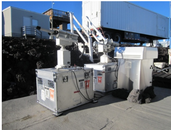
Standard sky radiometer POM-02 is calibrated in MLO.
