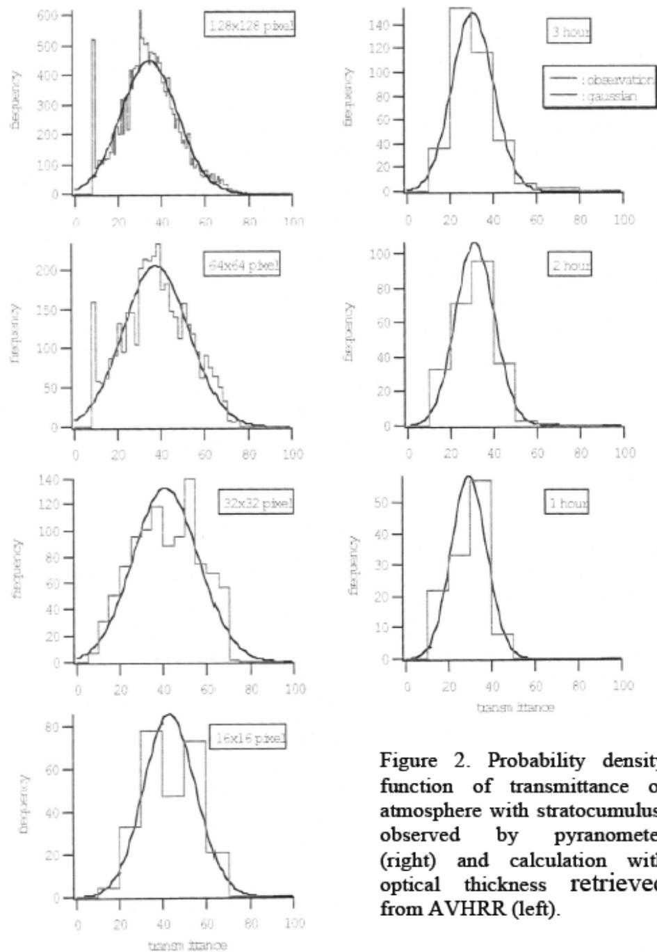
**Figure 2.** Probability density function of transmittance of atmosphere with stratocumulus, observed by pyranometer (right) and calculation with optical thickness retrieved from AVHRR (left).
