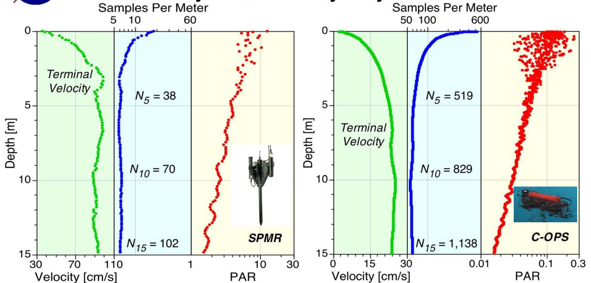
The buoyancy control enhancements to C-OPS result in an order of magnitude (or more) improvement in sampling resolution with respect to legacy instruments ( $N_z$  is the number of samples acquired by depth  $z$ , regardless of the tilt of the profiler). A noticeable consequence of the improved sampling resolution is a significant reduction in the aliasing of wave-focusing effects during clear-sky conditions.
