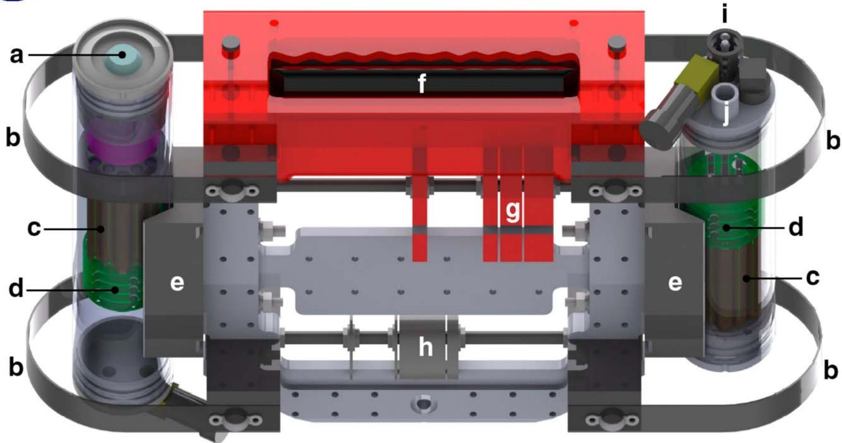
C-OPS uses 7 cm (OD) sensors: a) cosine collector; b) side bumpers; c) 19 microradiometers cluster; d) new compact aggregator; e) adjustable v-blocks counter pitch biases; f) hydrobaric buoyancy (compressible bladders) allows near-surface loitering; g) adjustable flotation counters roll biases; h) weights (and floats) set terminal velocity and; i) temperature probe and j) pressure transducer.
